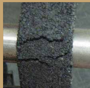
non-modified asphalt shingle with cracking
